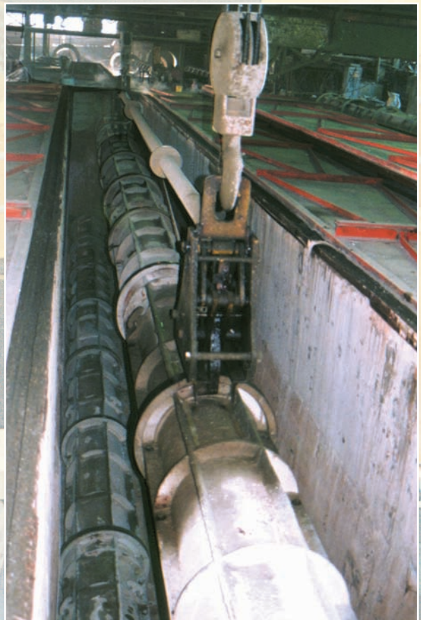
低溫養生槽 low-temperature curing chamber
