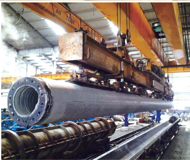
真空吸樁機(300-800) Vacuum lift for concrete pile (300~800)
