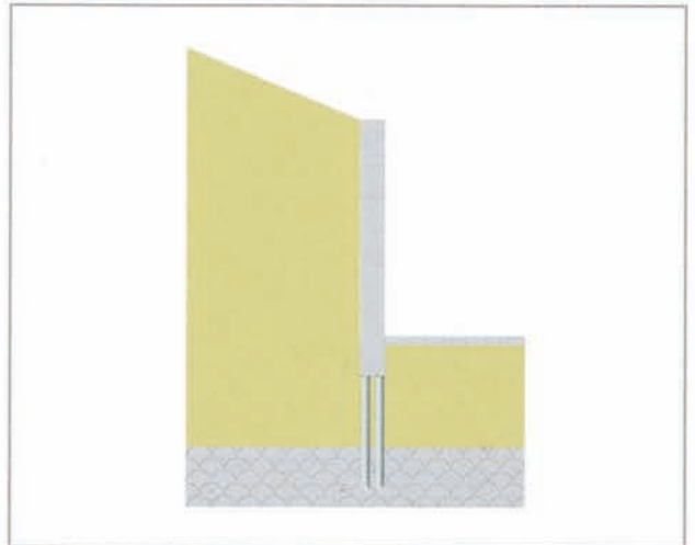
擋土牆 Retaining Wall
