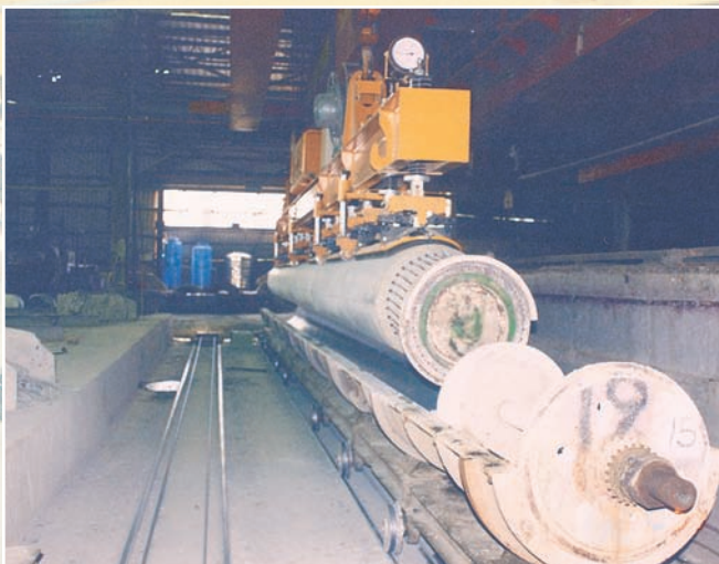
真空吸樁機(400~1000) Vacuum lift for concrete pile (400-1000)
