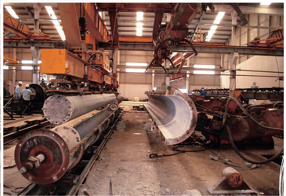
真空吸樁機 (300-800) Vacuum lift for concrete pile (300-800)
